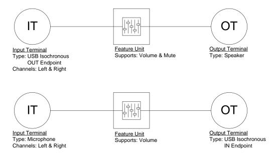
More complex audio devices are created by connecting multiple Unit entities together to describe the Device's capabilities. For more information about the available Unit and Terminal entities, and how they are used please refer to the USB Audio Class Device v1.0 specification.
